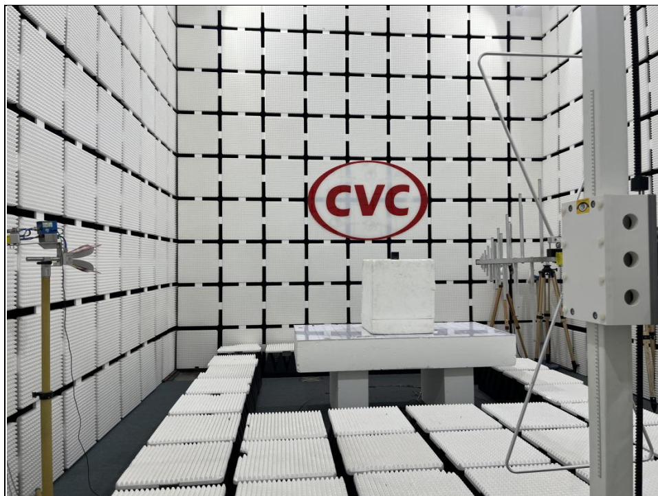
RADIATED SPURIOUS EMISSION TEST -1
