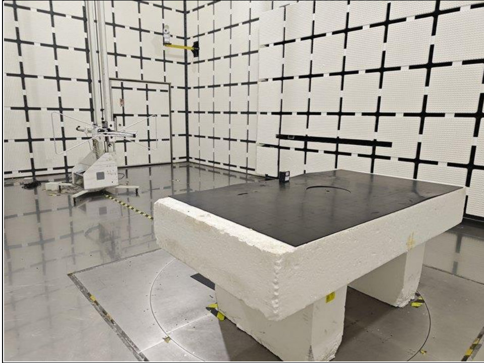
RADIATED EMISSION TEST BELOW 1GHz
