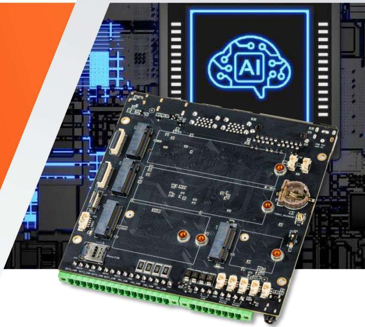
CamThink NG4500-CB01 is an extendable carrier board designed for the edge AI box NG4500 that requires differentiated computation power. The carrier board is compatible with NVIDIA® Jetson Orin™ Nano/NX platforms, and supports NVIDIA® Super Developer Kit, providing powerful edge AI computing capabilities. It is equipped with rich interfaces to simplify AI development and prototyping, suitable for application scenarios such as machine vision, industrial automation, robotics, and AIoT.
